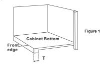
b) Fold the Mounting Template along the guideline that is closest to the thickness (see dimension "T" in illustration) of your cabinet overhang.
